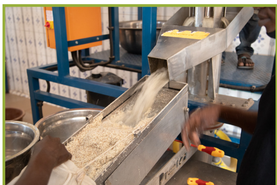
Figure 5: Fonio moving through the newly commissioned line
